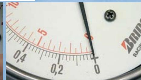
Turning the adjusting screw used for zeroing it, the needle can be put onto the zero on the device. This is what the needle position should be like after having adjusted it.
