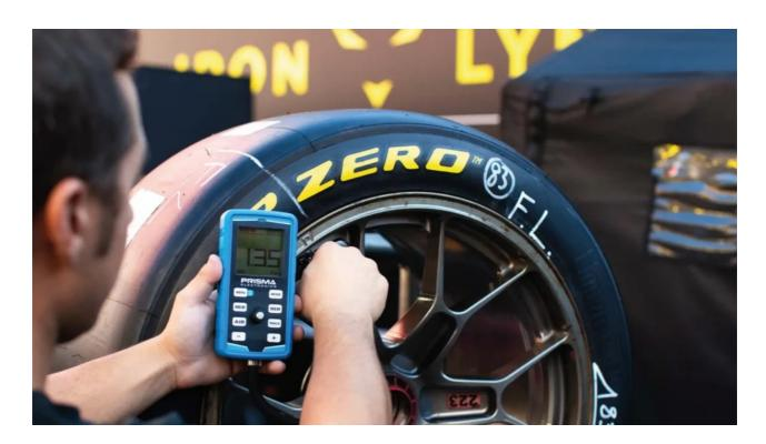
Therefore, it is crucial in motorsport to utilize tyres within the correct temperature range to achieve maximum performance and minimize degradation.
